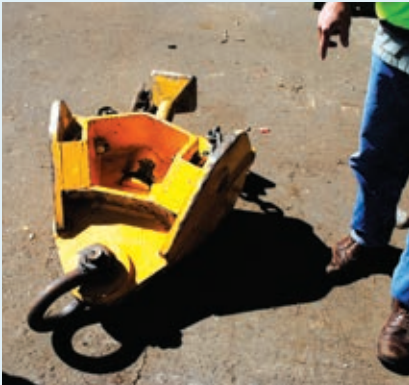
The self-releasing log head mechanism has reduced injuries at Oregon ports.
