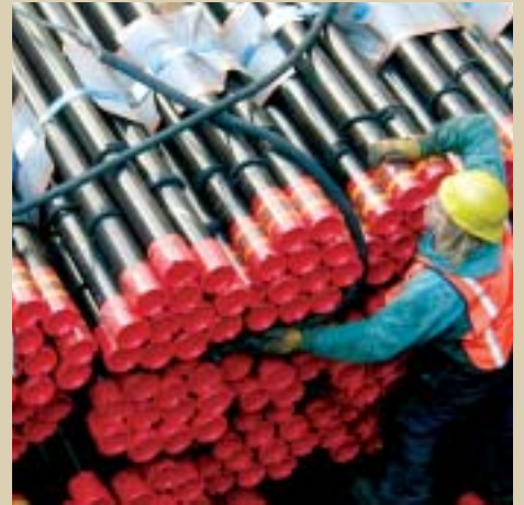
Rigging slings to prepare steel pipes from Japan for discharge.
