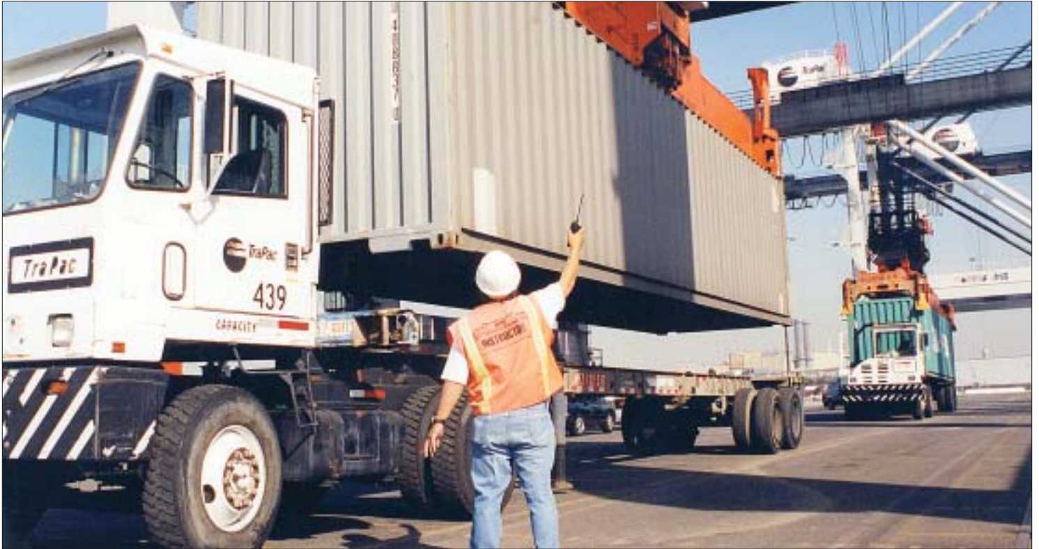
A Local 13 Crane Training Instructor coaches a trainee to float a container before landing on a chassis.
