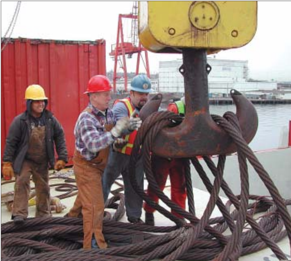
Longshore workers rig gear in order to discharge transformer from heavylift ship Tracer at SSA Terminals, Port of Seattle.
