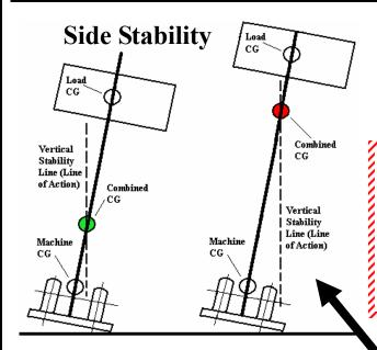
A Side Tip-over occurs when a turn is made with a weight lifted high in the air.
