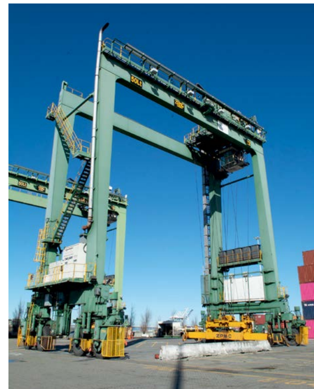
One of 13 retrofitted battery-powered hybrid gantry cranes.
