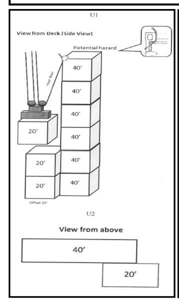
When on-deck 20' containers are stowed offset of an abreast 40' container stack the hoist ropes can align with corner castings. The slack hoist ropes can snag on the corner castings causing containers to be pulled down, this can also damage the integrity of the hoist ropes. Therefore, the following protocol shall be used:
